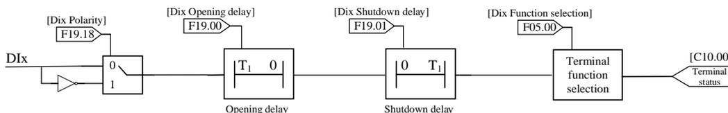
Figure 5-8 DI terminal processing
