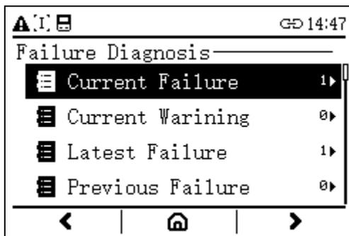
4. Enter the " Current Failure" to view the current fault information including fault codes and fault sub-codes.
