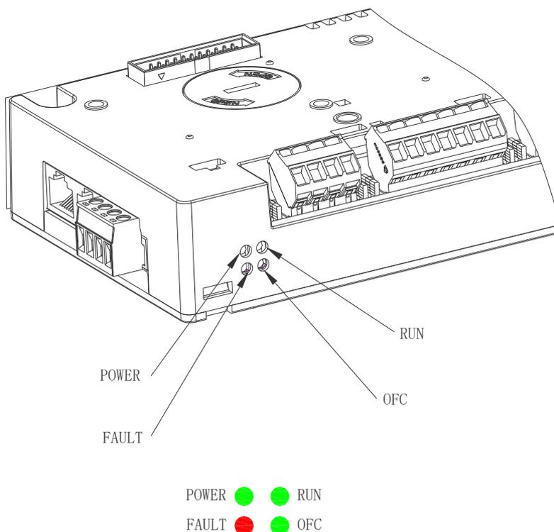
Figure 2-5 VF-400-CINU+DCDC indicator position
