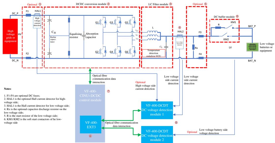
Figure 2-2 DC chopper device system topology diagram
