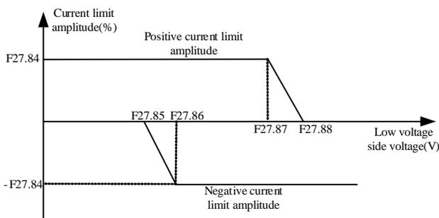
Figure 5-3 The LV-side overvoltage and undervoltage protection curve
