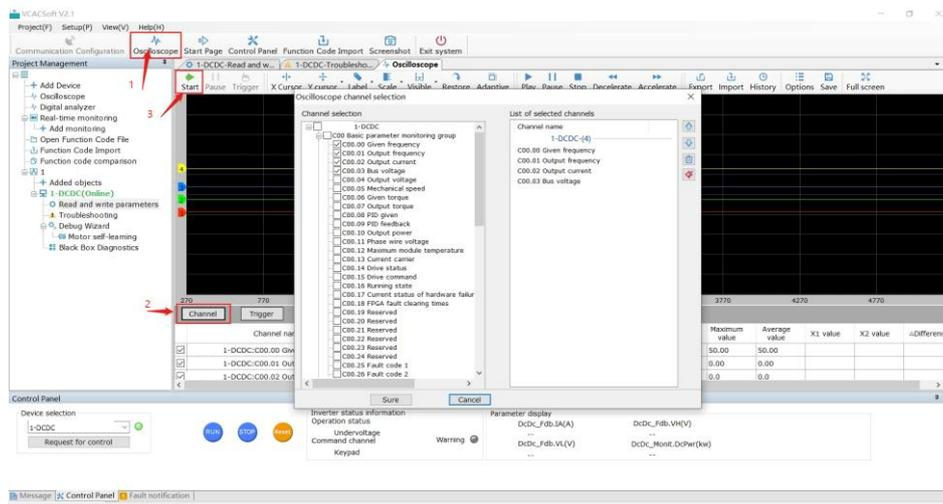
Figure 3-14 Continuous oscilloscope monitor interface
