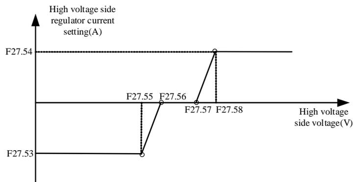
Figure 5-1 Relationship of HV-side voltage and HV-side regulator current
