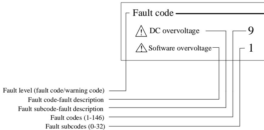
Figure 7-1 Fault code example
