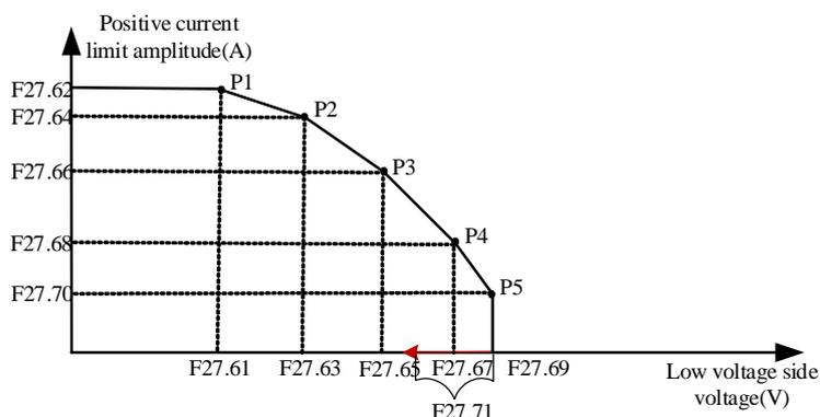
Figure 5-2 The relationship between LV-side voltage and positive current limit
