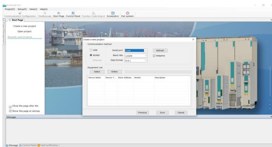
Figure 3-6 Set the communication method
