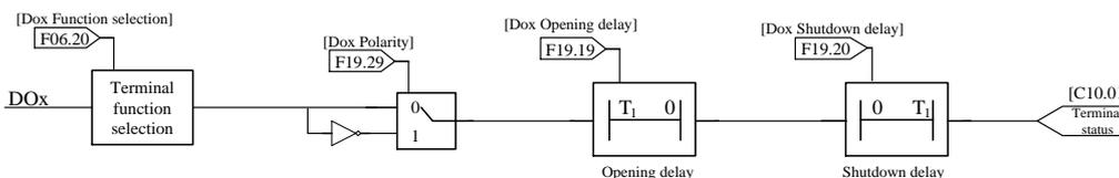
Figure 5-9 DO terminal processing
