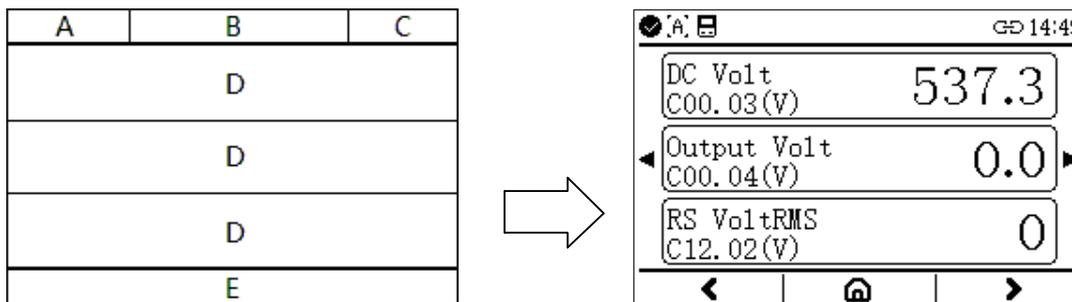
Figure 3-3 Display of the main monitoring interface under shutdown
