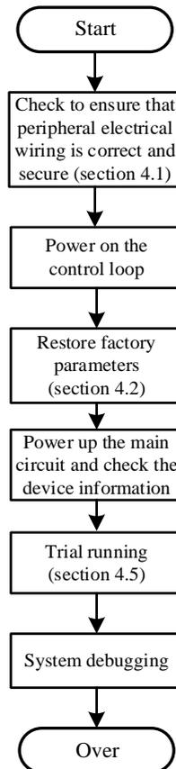
Figure 4-1 System debugging flowchart
