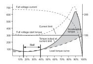
Start current can be estimated based on previous experience, or the motor and load speed/torque curves can be analysed for a precise calculation. A single soft starter can be used to control multiple motors, either in sequence or in parallel, provided the soft starter is correctly selected for the application.
