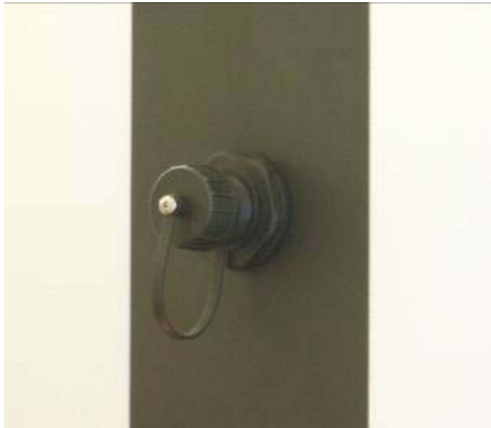
Figure 6. USB connector installed on door.
