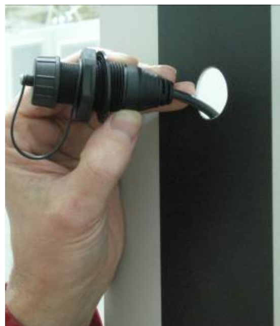
Figure 4. Inserting USB cable into feed-through hole.
