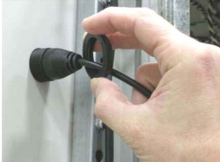
Figure 5. Securing USB connector with retaining nut.
