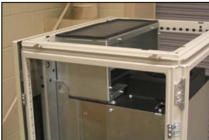
Figure 19. Top duct assembly installed
