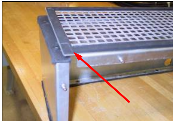
Figure 15. Gasket folds over the edge to form seal between the duct and top vented cover
