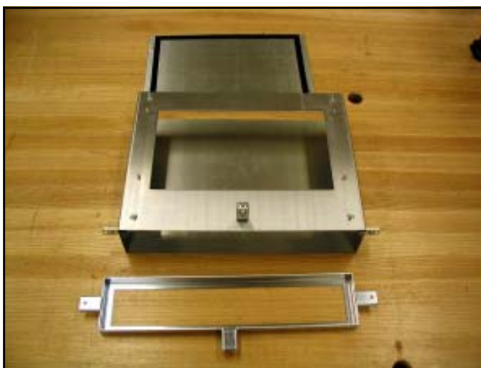
Figure 25. Bottom duct partially assembled
