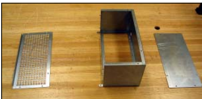
Figure 12. The top duct work partially assembled with bottom flange
