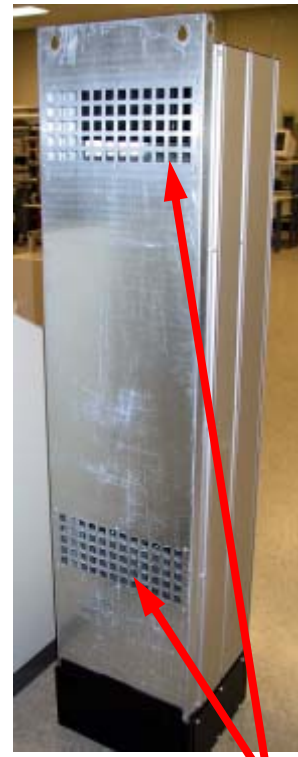
Photo 1. Drive openings on rear are not used in this application.
