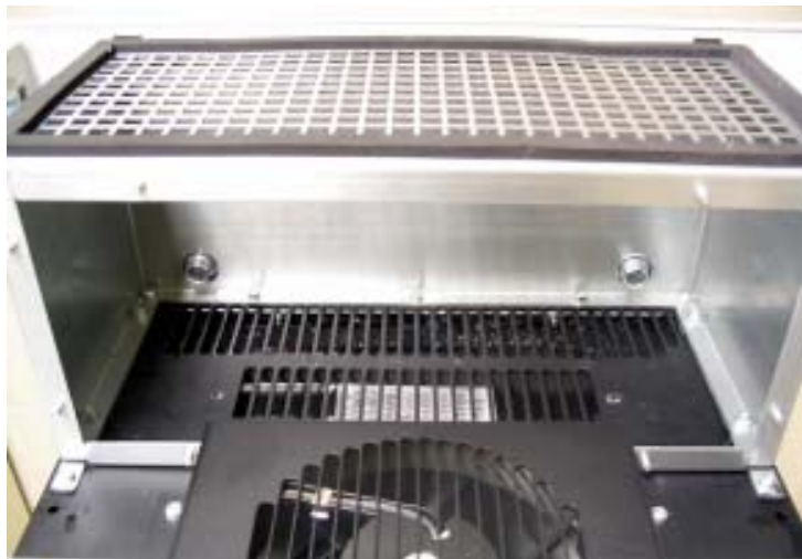
Photo 14. Top duct installed.
