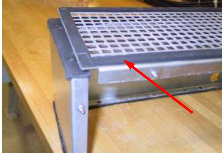
Photo 13. Gasket folds over the edge to form seal between the duct and top vented cover.
