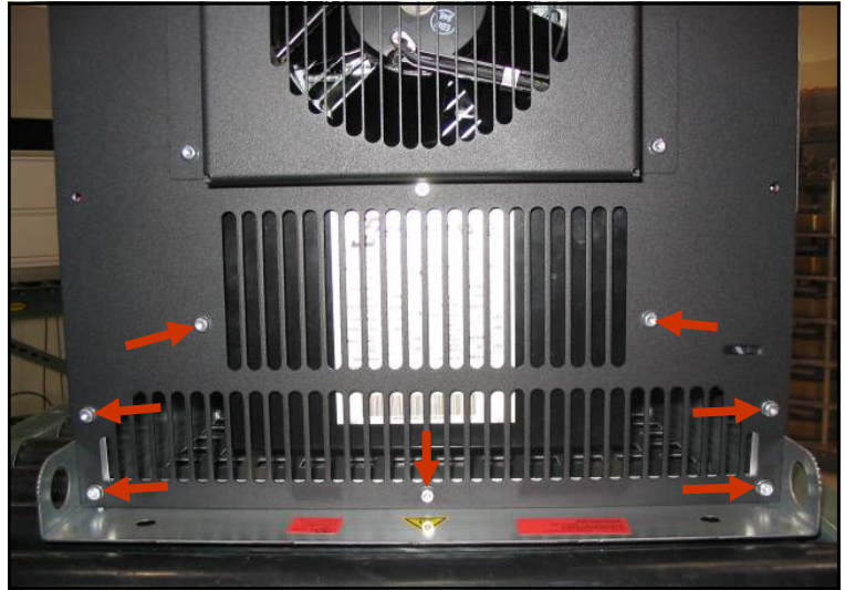
Figure 5. Screws to be removed from top of drive
