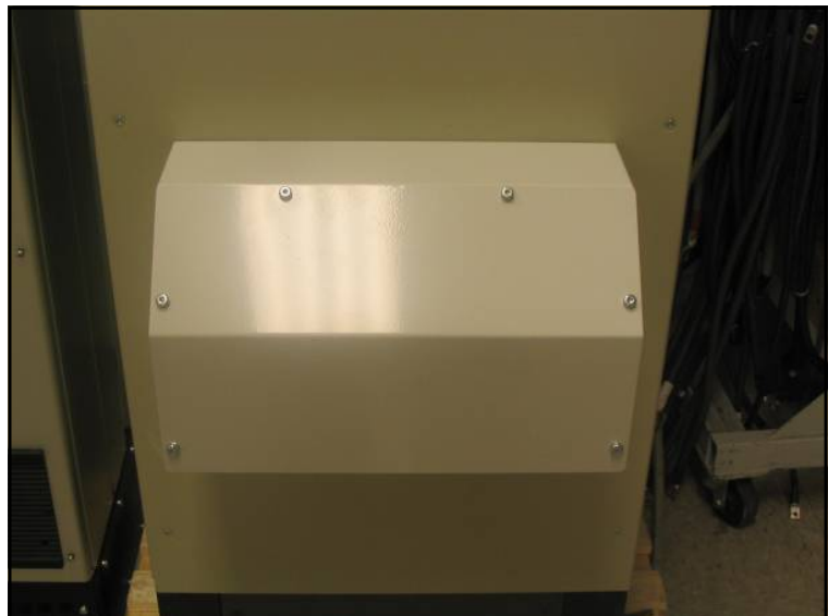
Figure 23. Lower deflector assembly installed
