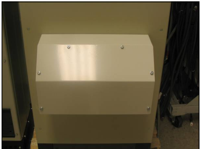
Figure 21. Lower deflector assembly installed
