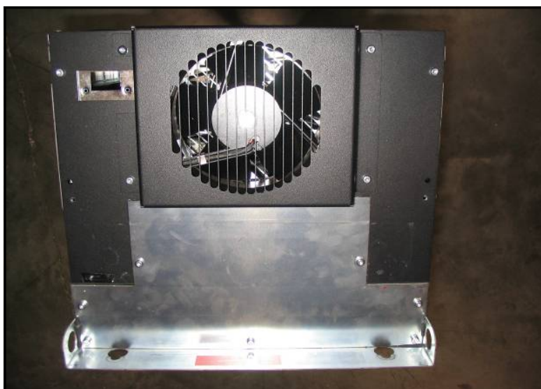
Figure 3. Top cover plate installed
