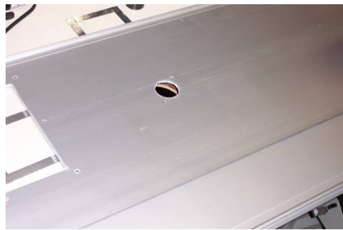
Photo 16. The shaft feed-through hole and the 5mm holes for mounting the handle.
