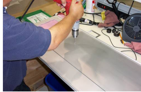
Photo 15. Drilling the 5mm holes for mounting the handle.
