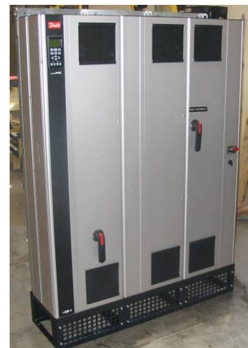
Photo 2. Tier 3 Frame D2 APU with pedestal
