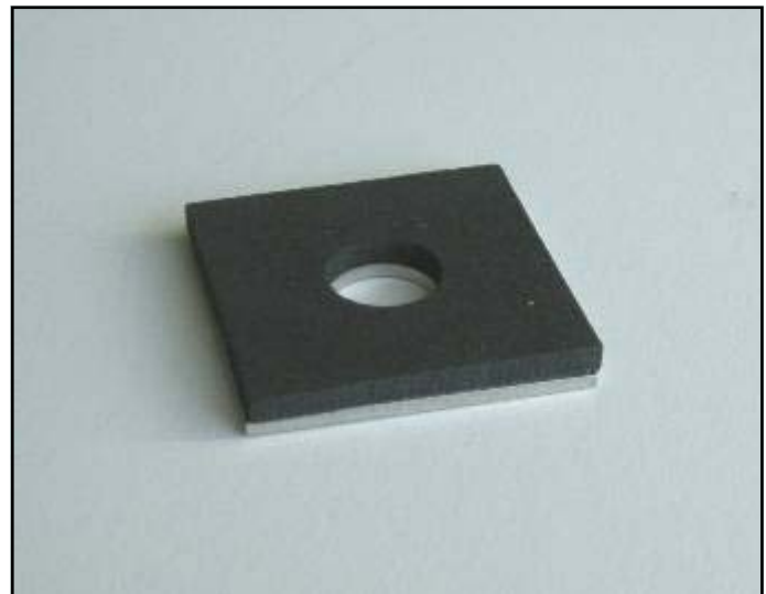
Figure 8. Gasket mounted on sealing plate
