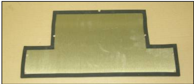
Figure 2. Gasket applied to top cover plate
