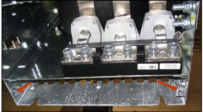
Figure 4. Bottom plate mounting brackets
