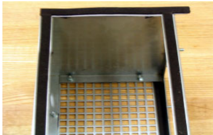
Photo 11. Gasket applied to both sides drive bracket and grated cover.
