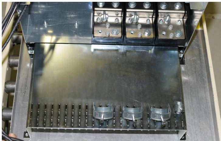
Figure 11. Cable-clamp bracket mounted on E2 frame.
