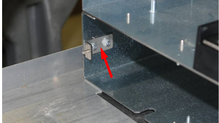
Figure 7. Mounting tab installed on left side of E2
