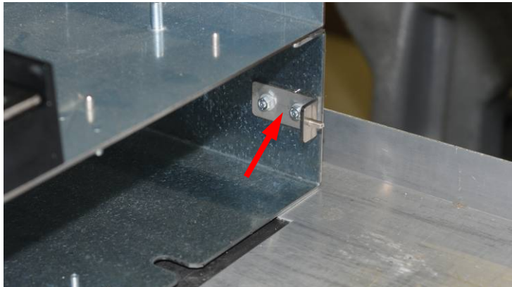
Figure 8. Mounting tab installed on right side of E2 frame.
