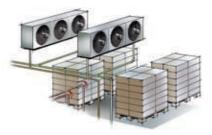
Reduced ice build-up and optimised evaporator temperature leads to lower energy consumption and higher system efficiency. The energy consumption is reduced by always matching capacity to the actual load.
