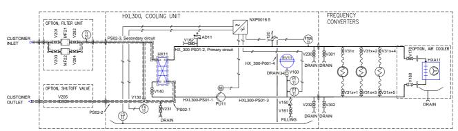
Figure 2.2-2 Piping and instrumentation diagram (P&ID)
