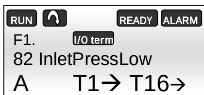
Figure 5.1-4, Low pressure alarm on the NXP panel
