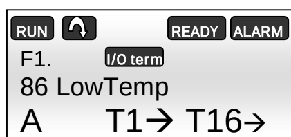
Figure 5.1-3, Low temperature alarm on the NXP panel
