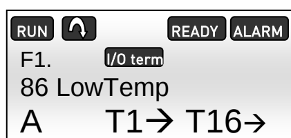
Figure 5.1-3, Low temperature alarm on the NXP panel
