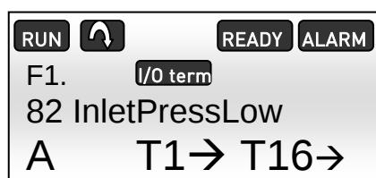
Figure 5.1-4, Low pressure alarm on the NXP panel
