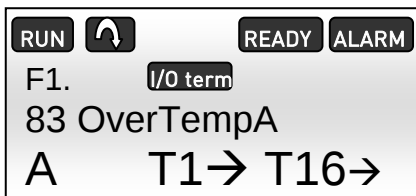
Figure 5.1-2, High temperature alarm on the NXP panel
