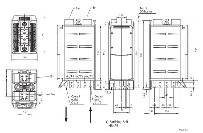
Figure 12. VACON® Liquid-Cooled inverter, CH61
