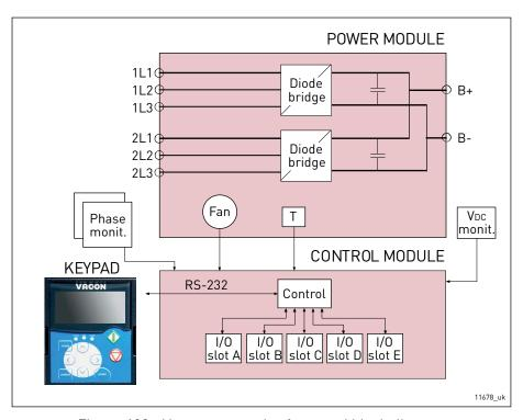
Figure 102. Non-regenerative front end block diagram
