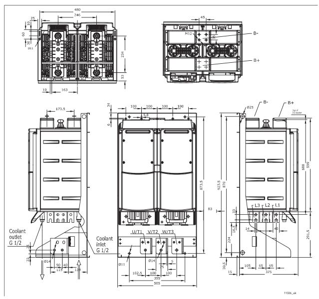
Figure 18.  $VACON^{\circledR}$  Liquid-Cooled AC drive with mounting bracket, CH63
