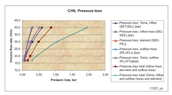
Figure 29. Pressure loss, CH6x
