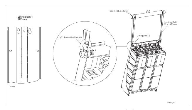
Figure 3. Lifting points for drives consisting of one module (left) and several modules
