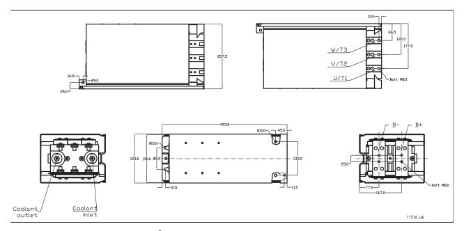
Figure 8. VACON® NX Liquid-Cooled drive dimensions (inverter), CH4
