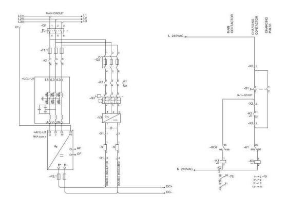
Figure 94. Wiring diagram for AFE unit
