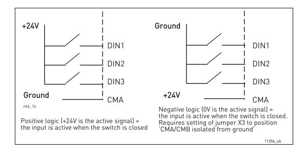
Figure 47. Positive/Negative logic
