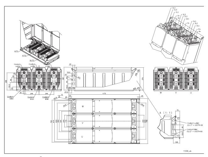
Figure 22. VACON $^{\otimes}$  NX Liquid-Cooled AC drive (6-pulse) with internal brake chopper dimensions, CH74, IP00
