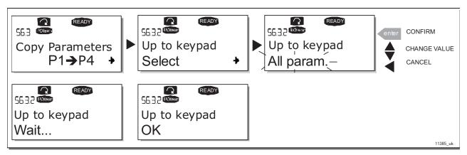
Figure 71. Parameter copy to keypad
