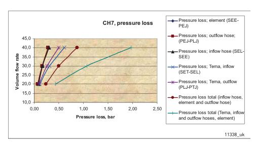
Figure 30. Pressure loss, CH7x
