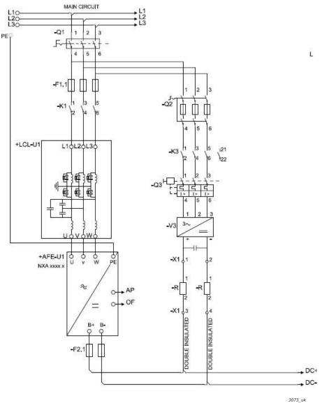
Figure 85. Active front end configuration
