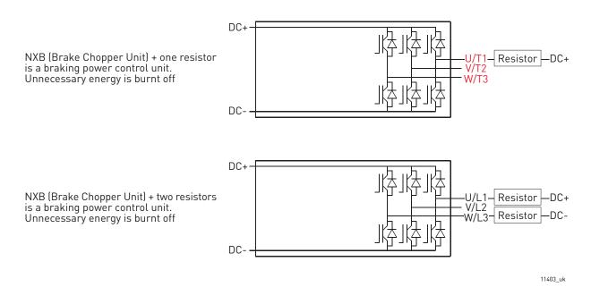
Figure 107. Brake chopper unit topology
