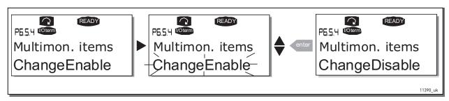
Figure 76. Enabling the change of multimonitoring items
