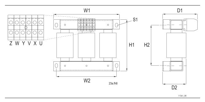
Figure 33. Example of input chokes for  $VACON^{\otimes}$  NX Liquid-Cooled. Sizes up to 62 A
