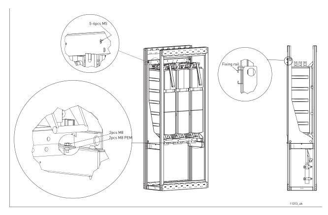
Figure 5. Securing the drive to the cabinet frame
