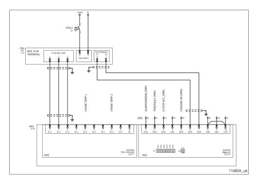
Figure 100. Wiring diagram for controls, OPTBH, OPTB1
