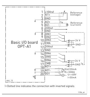
Figure 43. The I/O terminals of the two basic boards
