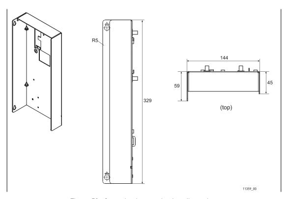
Figure 50. Control unit mounting box dimensions
