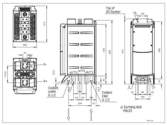
Figure 13. VACON® Liquid-Cooled inverter, CH62
