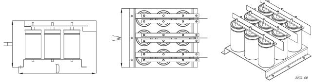
Figure 90. Example of capacitor bank ( $C_{bank}$ ) of a VACON $^{\circledR}$  RLC filter
