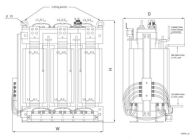
Figure 88. Example of  $L_{net}$  choke of a VACON<sup>®</sup> RLC filter
