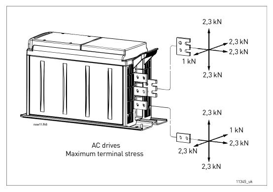
Figure 37. Maximum terminal stresses
