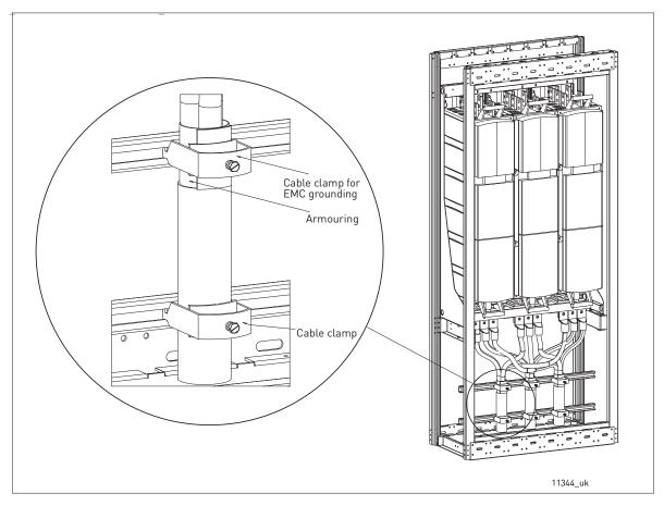
Figure 36. Clamping the motor cables to cabinet frame
