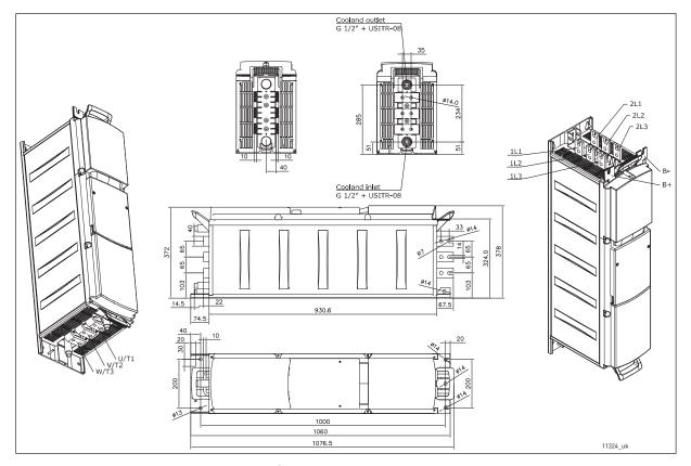
Figure 16.  $VACON^{\circledast}$  Liquid-Cooled AC drive (12-pulse), CH72
