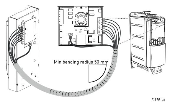
Figure 56. Connecting the power supply and control cables to the control unit, Ch6x
