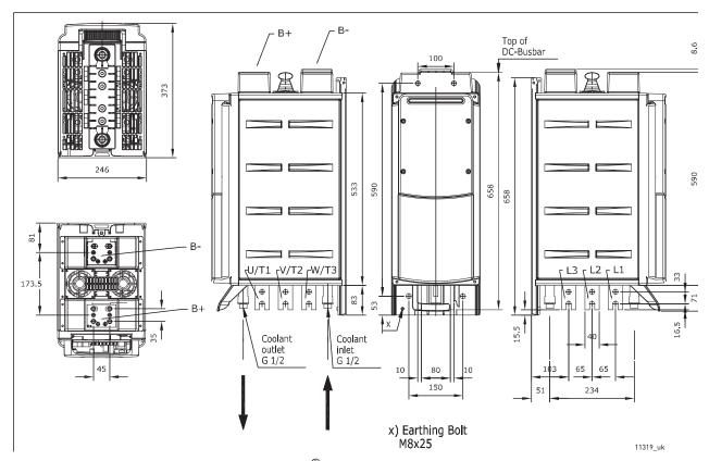
Figure 11. VACON® Liquid-Cooled AC drive, CH61
