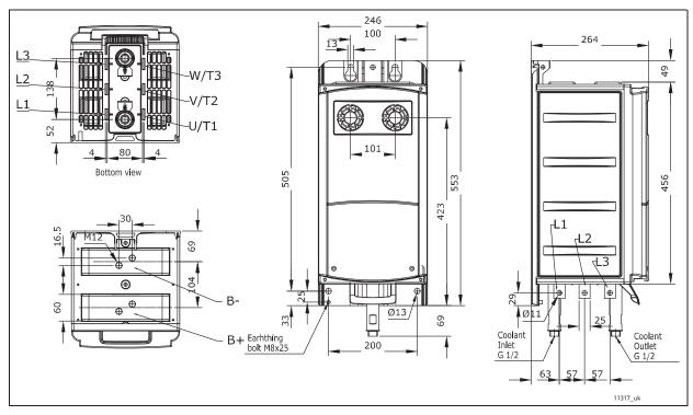
Figure 9. VACON® NX Liquid-Cooled dimensions, CH5 AC drive
