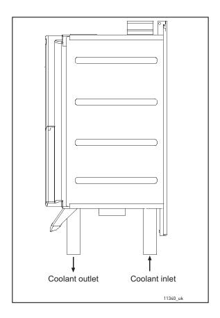
Figure 32. Direction of coolant circulation
