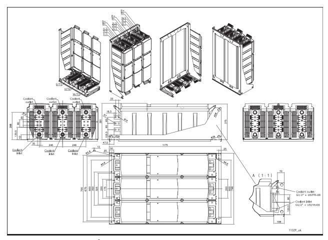
Figure 21. VACON® NX Liquid-Cooled AC drive (6-pulse) dimensions, CH74, IP00
