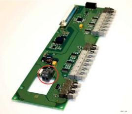
The control board can also be powered externally  $(+24 \text{ V}, \pm 10\%)$  by connecting the external power source to either of the bidirectional terminal #6 or #12, see page 98.
