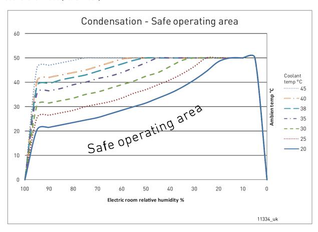
Figure 26. Safe operating conditions in relation to condensation
