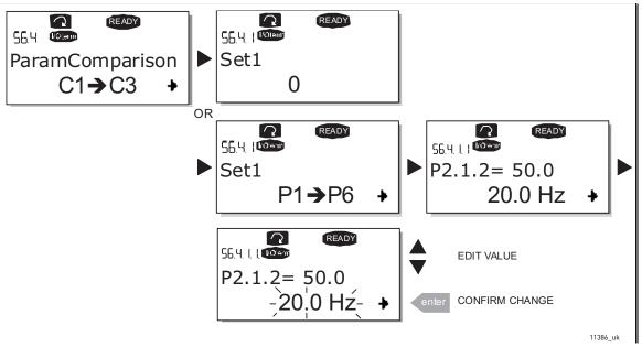
Figure 72. Parameter comparison
