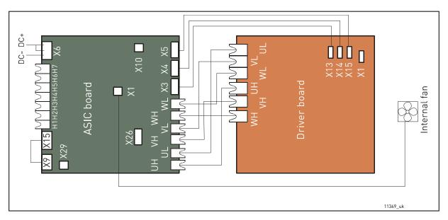
Figure 52. Terminals and connections between ASIC and driver board (CH61, CH62 and CH72)
