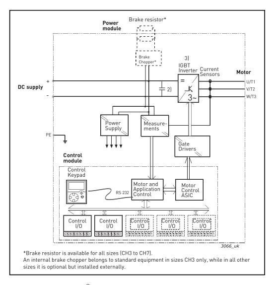
Figure 2. VACON® NX Liquid-Cooled inverter principal block diagram
