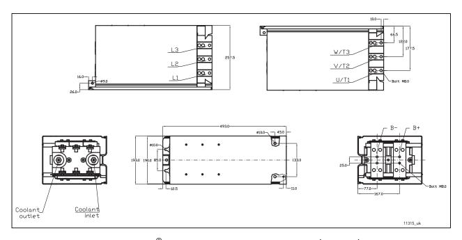
Figure 7. VACON® NX Liquid-Cooled drive dimensions (AC drive), CH4
