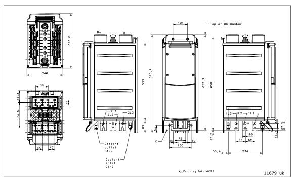
$\overline{\hspace{0.2cm}}$  Figure 103. VACON $^{ ext{ iny B}}$  Liquid-cooled Non-regenerative front end, CH60
