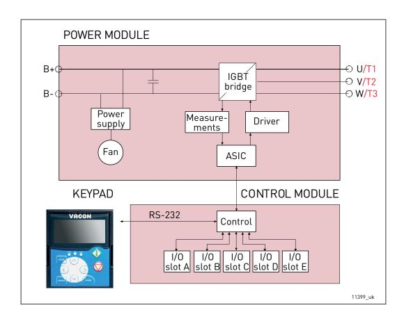
Figure 86. Active front end block diagram
