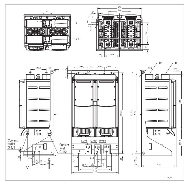
Figure 19. VACON® Liquid-Cooled inverter with mounting bracket, CH63
