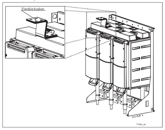
Figure 38. Mounting of flexible busbar
