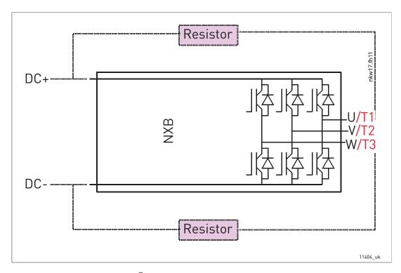
Figure 108. VACON® Brake Chopper Unit connections
