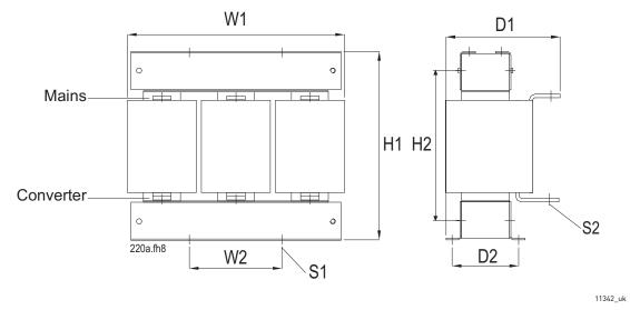
Figure 34. Example of input chokes for  $VACON^{\otimes}$  NX Liquid-Cooled. Sizes 87 A... 145 A and 590 A
