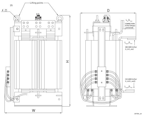
Figure 89. Example of  $L_{afe}$  choke of a VACON<sup>®</sup> RLC filter
