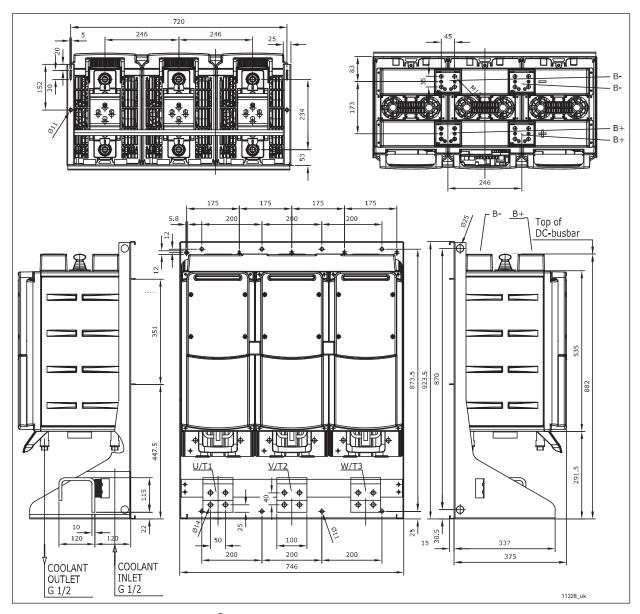
Figure 20. VACON® NX Liquid-Cooled inverter dimensions, CH64, IP00
