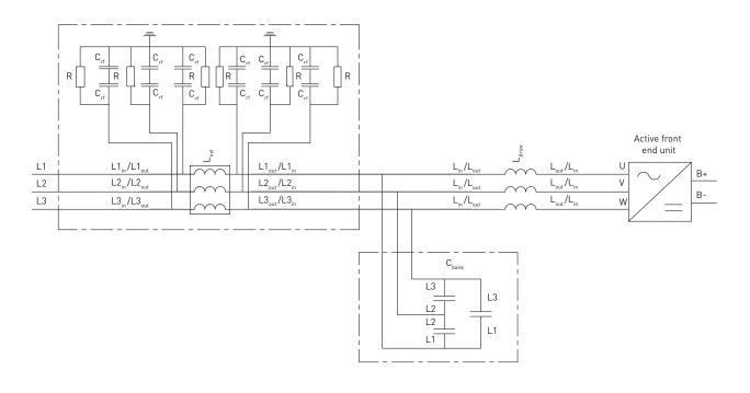
Figure 87. VACON® RLC filter wiring diagram
