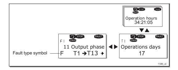
Figure 66. Fault display
