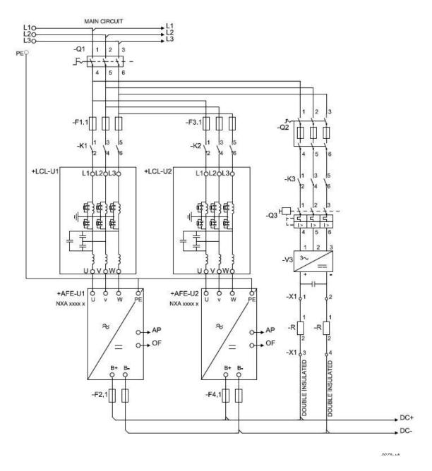
Figure 96. Active Front End units parallel connection with one common pre-charging circuit
