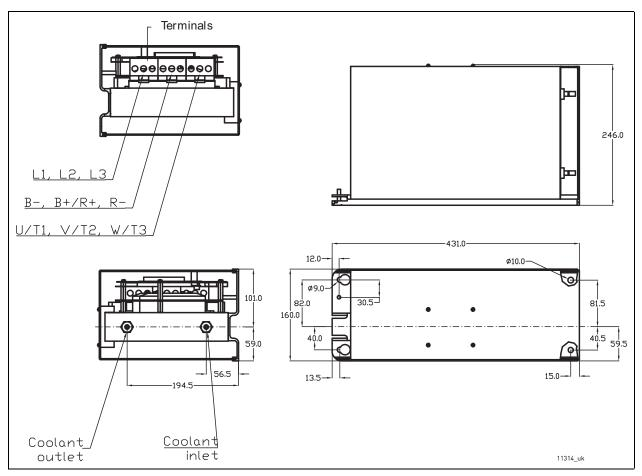
Figure 6.  $VACON^{\circledR}$  NX Liquid-Cooled drive dimensions, CH3
