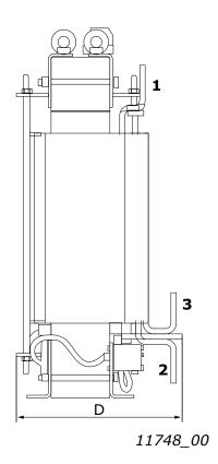
Figure 105. Example of FLU-CHK-1030-6-DL choke
