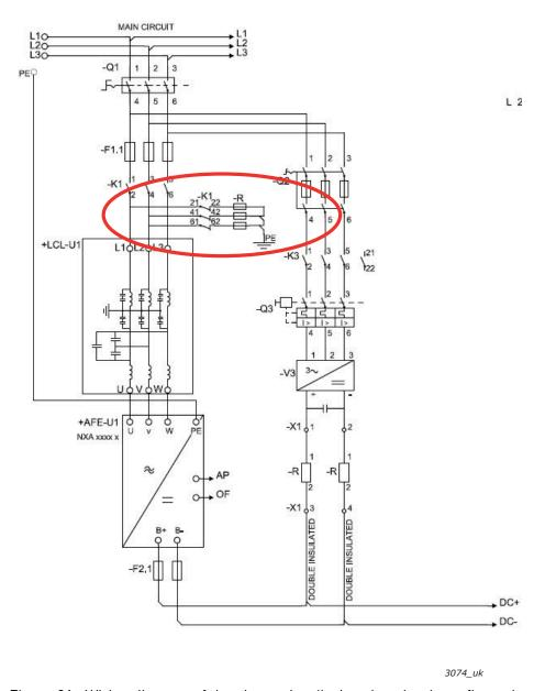
Figure 91. Wiring diagram of the alternative discharging circuit configuration
