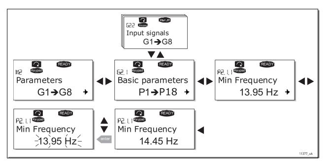
Figure 64. Parameter value change procedure
