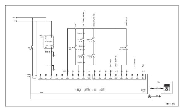
Figure 99. Wiring diagram for controls, OPTA1.
