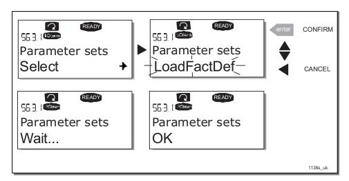
Figure 70. Storing and loading of parameter sets
