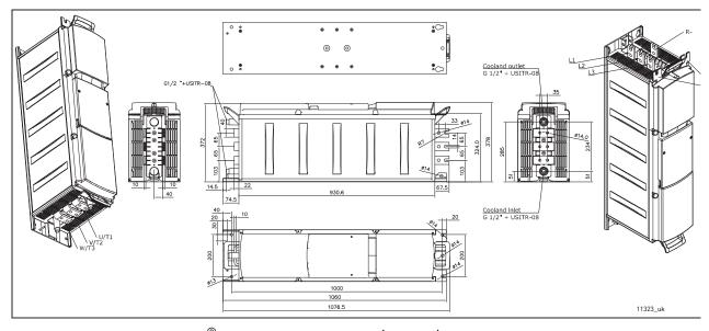
Figure 15. VACON® Liquid-Cooled AC drive (6-pulse) with internal brake chopper
