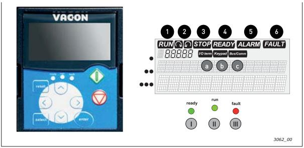
Figure 60. VACON® control keypad and drive status indications
