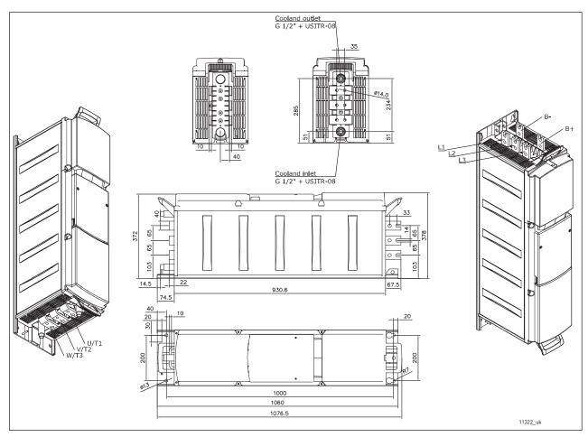
Figure 14. VACON® Liquid-Cooled AC drive (6-pulse), CH72
