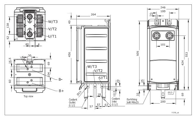
Figure 10. VACON® NX Liquid-Cooled dimensions, CH5 inverter
