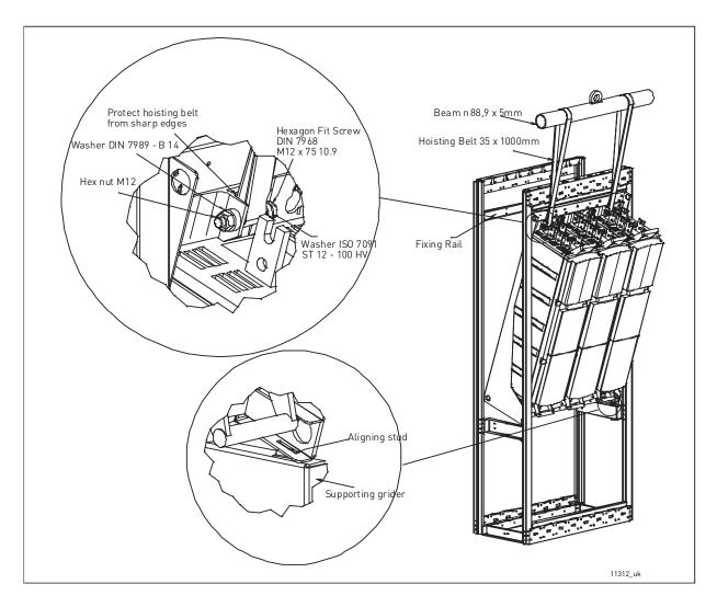
Figure 4. Lifting of drive into a narrow mounting space
