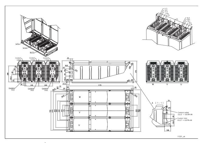
Figure 23. VACON  $^{\otimes}$  NX Liquid-Cooled AC drive (12-pulse) with internal brake chopper dimensions, CH74, IP00
