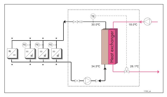
Figure 24. Example of cooling system
