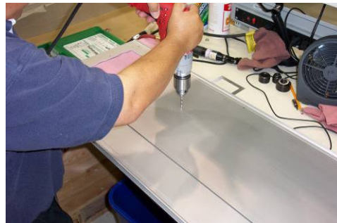
Photo 15. Drilling the 5mm holes for mounting the handle.
