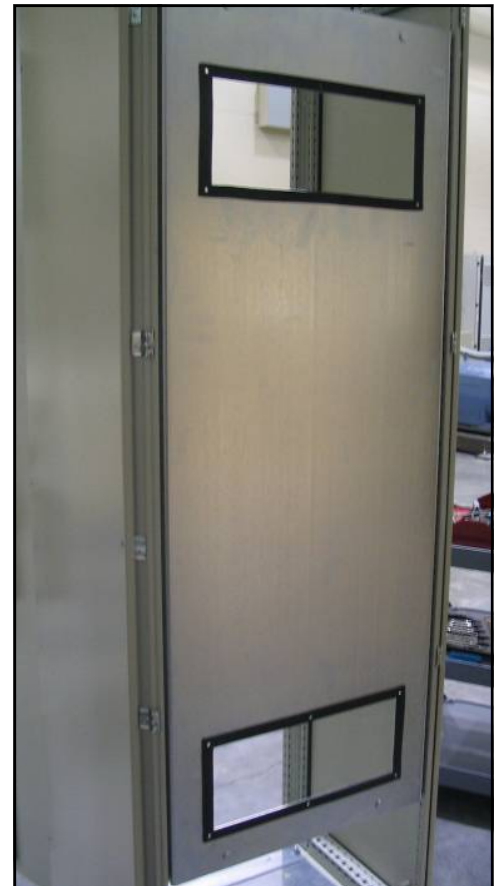
Figure 8. Back of drive mounting plate with gasket installed
