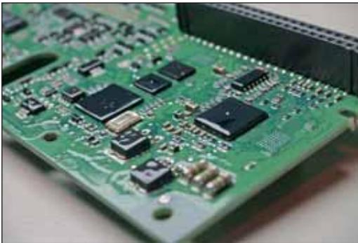
*Fig. 9.8 Printed circuit board with conformal coated*
